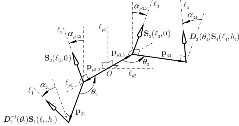
**Fig. 6** Quaternary generator of a 4-PSS with a constant class of the general type.
