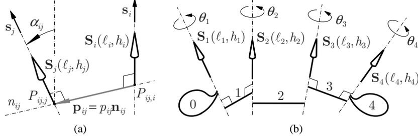
**Fig. 1** Relative pose between two screws (a); a chain of four 1-dof lower pairs (b).
