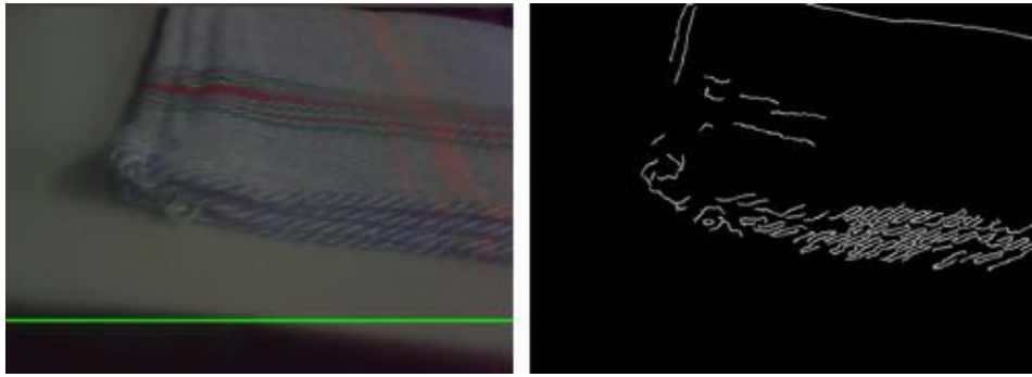
Figure 26: Example of Canny segmentation on the image of a textured cloth
