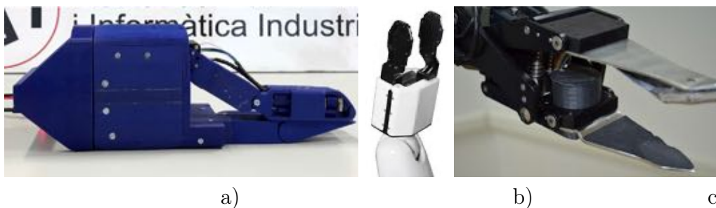
Figure 4: Examples of rigid grippers. a) gripper designed at Institut de Robòtica i Informàtica Industrial in Barcelona [25], b) gripper designed by Pal Robotics for TIAGo robot [26], c) gripper designed by Information Technology Institute in Thessaloniki [27].
