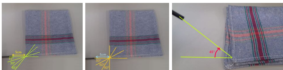
Figure 15: Setup of the tests with the textured cloth
