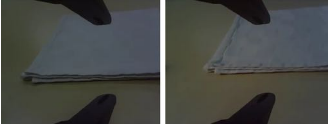
Figure 78: Different light conditions, 554-560lux on the left, 825-832lux on the right
