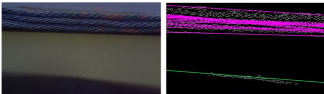
Figure 31: Hough lines on images of a textured cloth where has been applied only the Canny edge detector
