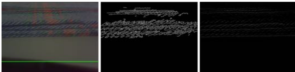
Figure 27: Original image of a textured cloth, effect of Canny edge detector, effect of Canny edge detector and Sobel filter
