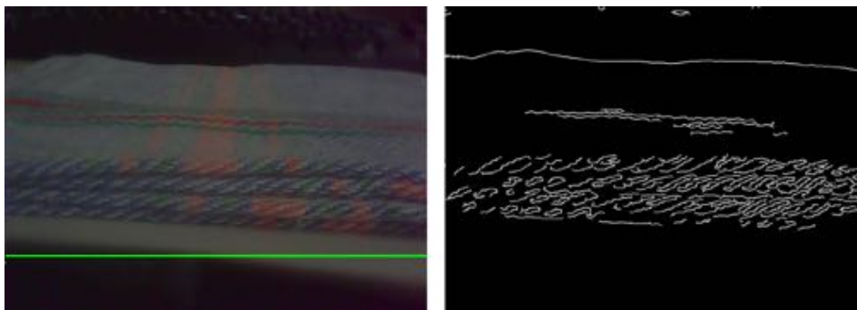
Figure 25: Example of Canny segmentation on the image of a textured cloth
