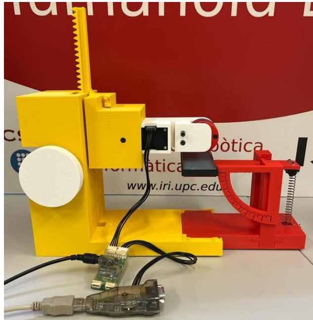
Figure 3.2.1.1: Image of the complete test-bench with the connections of the USB and Power adapters to the motor.
