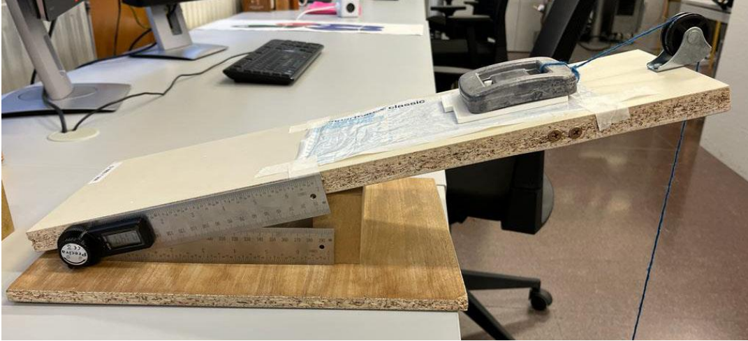
Figure 3.1.1: Photograph of the inclined plane constructed with the materials mentioned.
