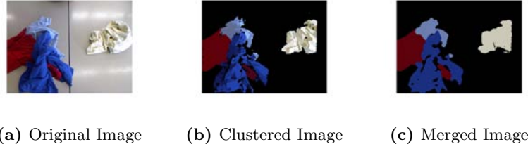
Figure 14 – Image segmentation output images at the three main steps of the proposed algorithm. The final count of objects would provide an observation of three objects on the left and one on the right.
