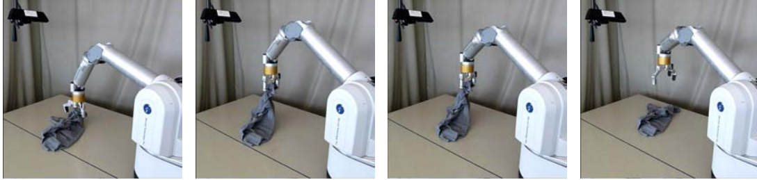
Figure 18 – Spreading sequence. Given a grasping point of the cloth, it is displaced to a peripheral point of the working area.
