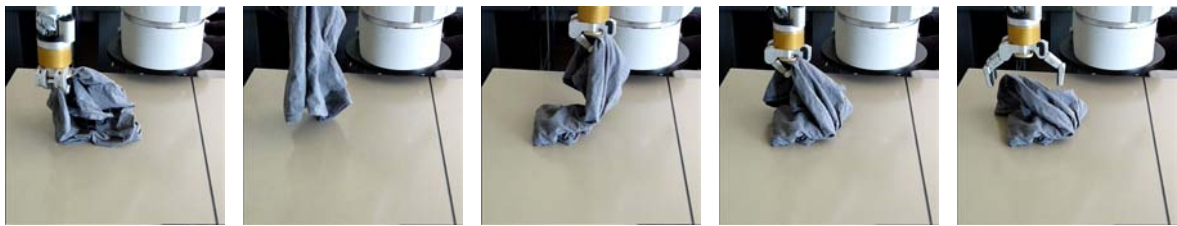
Figure 17 – Folding sequence. Since we are using a single manipulator, the table friction is used to fold the piece of cloth.
