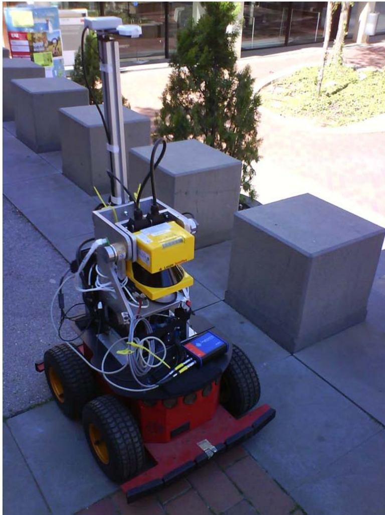
Figure 3.3: 3D laser range finder mounted on our robotic platform.
