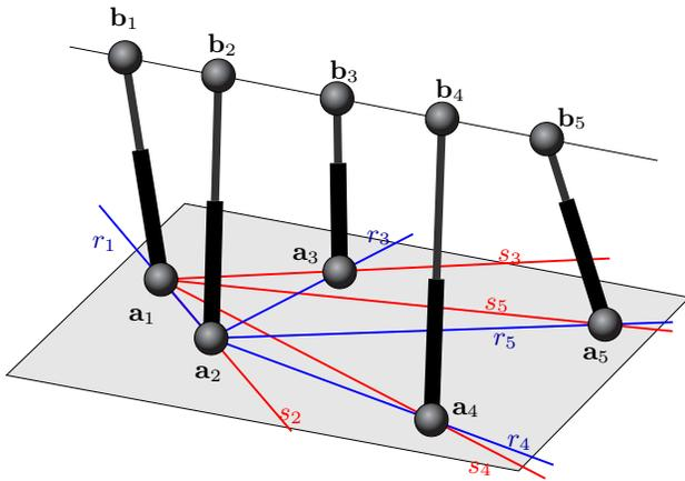
Fig. 3. A line-plane subassembly is architecturally singular if, and only if,  $CR(\mathbf{b}_2, \mathbf{b}_3, \mathbf{b}_4, \mathbf{b}_5) = CR_l(s_2, s_3, s_4, s_5)$  and  $CR(\mathbf{b}_1, \mathbf{b}_3, \mathbf{b}_4, \mathbf{b}_5) = CR_l(r_1, r_3, r_4, r_5)$ . By permuting indices, up to ten equivalent sets of conditions can be derived.
