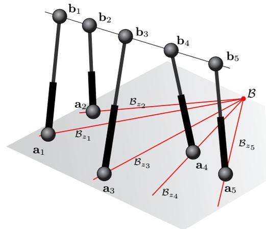
Fig. 4. The one-to-one correspondence between the attachments in the line and the lines of the pencil centered at  $B$ . Each value of  $z_i$  defines a point in the line,  $\mathbf{b}_i = \mathbf{p} + z_i\mathbf{i}$ , and a line in the plane  $B_{z_i}$ .
