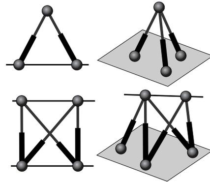
Fig. 1. Four rigid subassemblies involving linear geometric elements.
