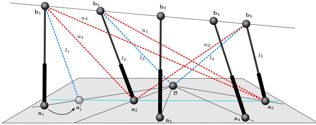
Fig. 7. The forward kinematics of a line-plane subassembly can be fully formulated in terms of distances.  $l_1$ ,  $l_3$  and  $l_4$  can be computed using the distance formula presented in Section V. Then,  $u_i$ , for  $i = 1, \dots, 4$  can be obtained using standard Distance Geometry techniques.
