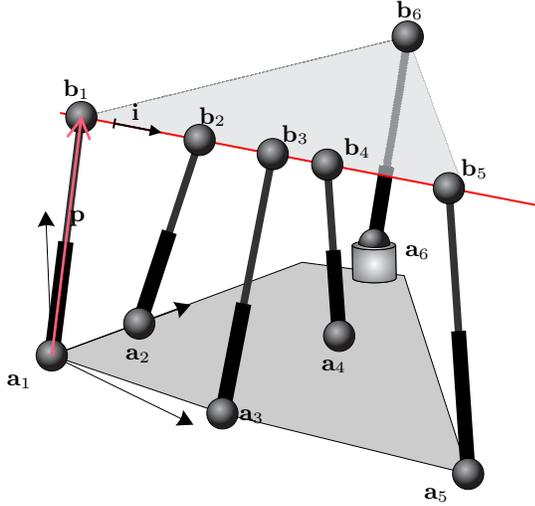
Fig. 2. Stewart platform containing a line-plane subassembly.
