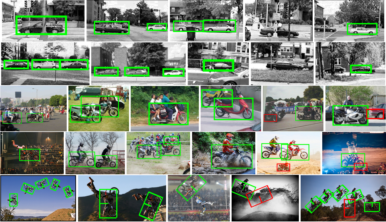
Figure 8. Detection results for different datasets. First row: UIUC multi-scale. Second row: UIUC single scale. Third row: TUD motorbikes. Fourth row: Freestyle motocross (Test 1). Fifth row: Freestyle motocross with in-plane rotations (Test 2).
