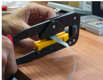
(a) Crimp tool to build the flat wire between the BLP and the BLL board.
