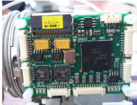
Figure 25: Detail of the board to control up to 2 brushless motors.
