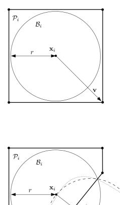
Figure 4: Progressive refinement of the applicability area of a chart of a 2D manifold. **Top** The applicability area,  $\mathcal{P}_i$ , of chart  $\mathcal{C}_i$  is initialized as a box including a ball of radius r around  $\mathbf{x}_i$ . **Bottom** The polytope is refined using a ball  $\hat{\mathcal{B}}_i^j$  that approximates  $\hat{\mathcal{C}}_i^j$ , the projection of a the area of the manifold covered by a neighboring chart into the current chart.
