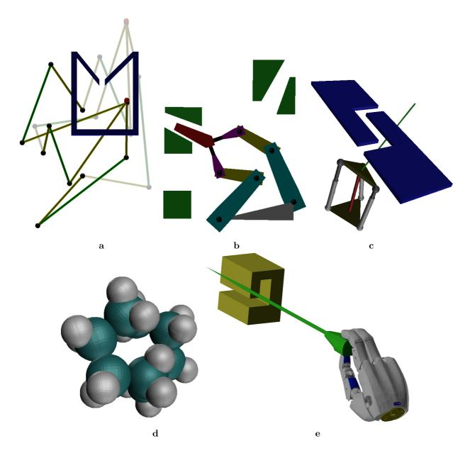
Figure 7: The five benchmarks used in the experiments. **a** A star-shaped planar manipulator with three fixed extremities and a bug trap like obstacle. **b** A two-arms manipulator moving an object from one gap to another. **c** A rotational-only parallel manipulator moving a stick among some obstacles. **d** The cyclooctane molecule. **e** The Schunk anthropomorphic hand performing an insertion task.
