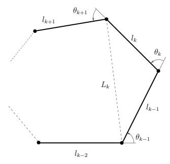
Figure 1: A single-loop planar linkage with revolute joints.
