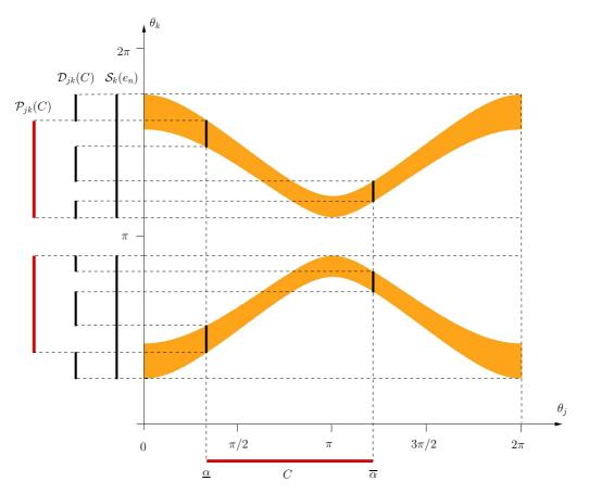
Figure 4: Propagation of interval  $C = [\underline{\alpha}, \overline{\alpha}]$  from  $\theta_j$  to  $\theta_k$ , obtaining  $\mathcal{P}_{jk}(C)$ .
