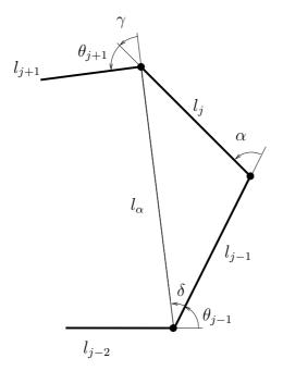
Figure 2: Substitution of variable  $\theta_j$  by a constant value  $\alpha$ .
