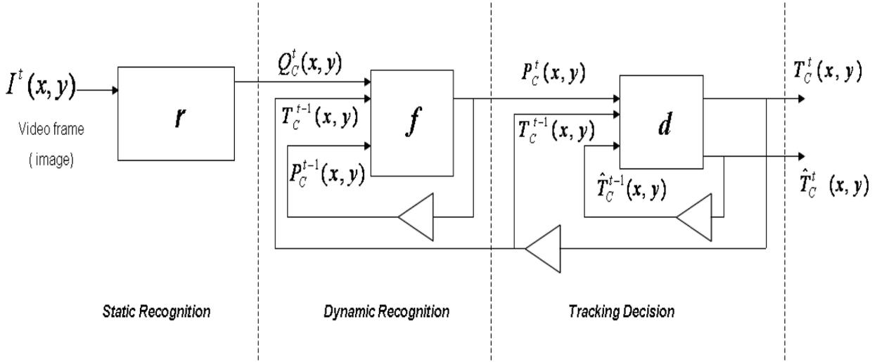
Figure 1: Block diagram of the dynamic object recognition and tracking process.
