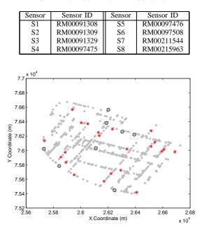
Fig. 3. DMA network with the optimal sensor location (black  $\circ$  symbol) and the remaining candidate sensors (red \* symbol)
