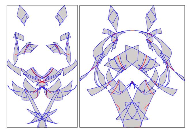
Figure 12: Output portraits of the manipulator in Fig. 11 assuming the geometric parameters mentioned in the text. The angles  $\theta_1$  and  $\theta_2$  are limited by keeping their cosines to the ranges [0.5, 0.7] (left plot) and [0.6, 0.8] (right plot), with positive sines in both cases. Red and blue curves correspond to forward and inverse singularities, respectively.
