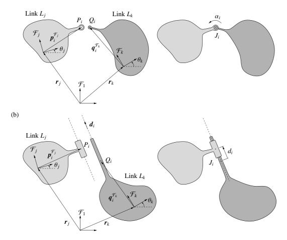
Figure 3: Geometric elements intervening in the assembly of revolute and prismatic pairs.
