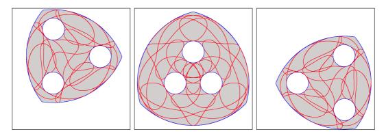
Figure 10: Slices of the output portrait of the 3-<u>R</u>RR manipulator computed by the method at fixed orientations of the platform, assuming the geometric parameters in Table 1, bottom. From left to right, the values  $\theta = -\frac{\pi}{4}$ , 0 and  $\frac{\pi}{4}$  are assumed. The plot of the  $\theta = 0$  slice agrees with the one published in [37, 16].
