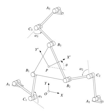
Figure 7: A planar 3-RR manipulator. Points  $A_1$ ,  $A_2$ , and  $A_3$  are fixed to the ground. Absolute (*OXY*) and relative (*PX'Y'*) reference frames are defined, fixed to the ground and to the moving platform respectively. The platform pose is given by the absolute coordinates (*x*, *y*) of a point *P*, and by the angle  $\theta$  of *PX'Y'* relative to *OXY*.
