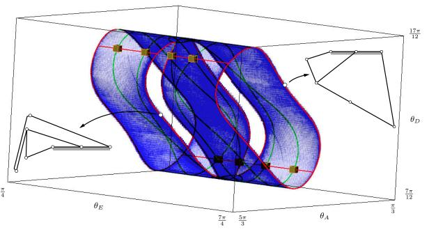
Fig. 9. A projection of the configuration space and the computed singularities to the  $(\theta_A, \theta_E, \theta_D)$  space, together with two configurations where C, G, and F are aligned. Green corresponds to the RI and IO types, red to the RO and II types, and orange to the RPM type. There are no singularities of IIM type.
