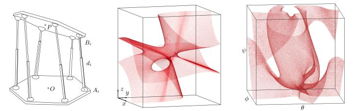
Fig. 11. Left: The Stewart-Gough platform. Center and right: Slices of its forward singularity set for a constant orientation given by  $\phi = -2^{\circ}$ ,  $\theta = 30^{\circ}$ , and  $\psi = -87^{\circ}$ , and for the fixed position  $p^{\mathcal{F}_1} = [10, 10, 10]^{\mathsf{T}}$ . The position and orientation variables of the platform have been limited to the ranges [-100, 100] and  $[-90^{\circ}, 90^{\circ}]$  respectively.
