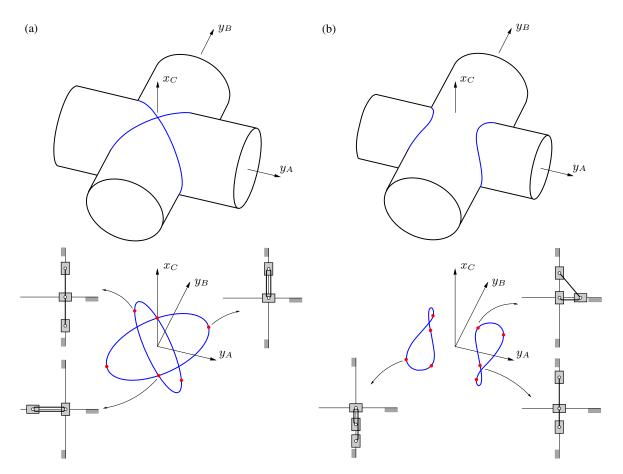
Fig. 2. Configuration space (in blue) and singularities (red dots) of the 3-slider mechanism for  $L_1 = L_2$  (a) and  $L_1 > L_2$  (b) with some examples of singular configurations depicted. In this mechanism, the configuration space corresponds to the intersection of two cylinders at right angles.
