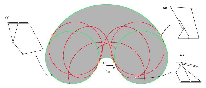
Fig. 8. A projection of the plot in Fig. 7 to the (x, y) plane. (a) A singularity of RPM, IO, and II type. (b) A singularity of RI and IO type. (c) A singularity of RO and II type.
