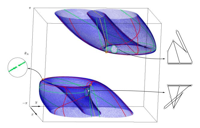
Fig. 7. The singular configurations of the mechanism in Fig. 5 shown overlaid onto a projection of its configuration space. Different colors are used to identify the several singularity types encountered: green for the RI, and IO types, red for the RO and II types, and orange for the RPM type.
