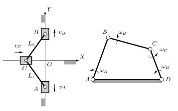
Fig. 1. Left: A 1-DOF mechanism with three sliders. The prismatic joints at A and B are on a line perpendicular to the axis of the prismatic joint at C. Right: A 4-bar mechanism. The angular velocities indicated refer to relative motions, e.g.,  $\omega_B$  is the angular velocity of link BC relative to link AB.
