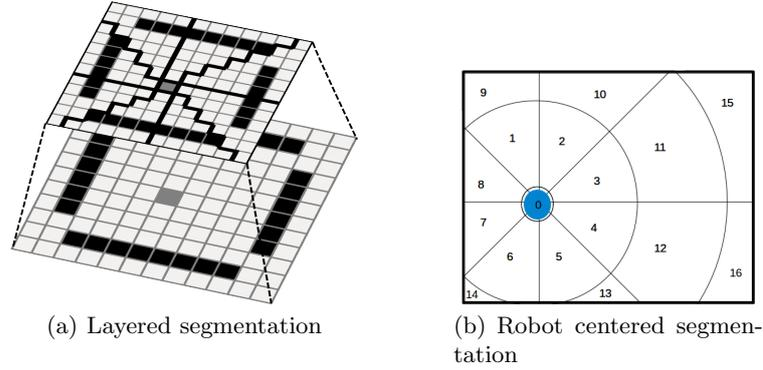
**Fig. 1.** The hierarchical method with two layers is shown in (a), where the top layer has less states due to segmentation of the lower level map. The *robot centered* segmentation (b) centers on the robot's location (0 in the figure) and from there on creates segments based on the direction and distance.
