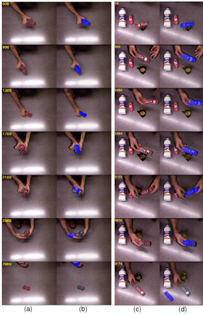
Fig. 5. Comparison of ((a) and (c)) our tracker (red rectangle) with ((b) and (d)) the tracker available in the Point Cloud Library (blue pixels). The color images are shown here for illustration only and not used in the tracking procedure. More results are provided in the accompanying video.
