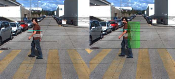
Figure 6: Example of detection using fusion with temporal information. Left Image, image without the temporal information used as feedback. Right image, image with the temporal information used as feedback. The right image shows that the person has been correctly detected.
