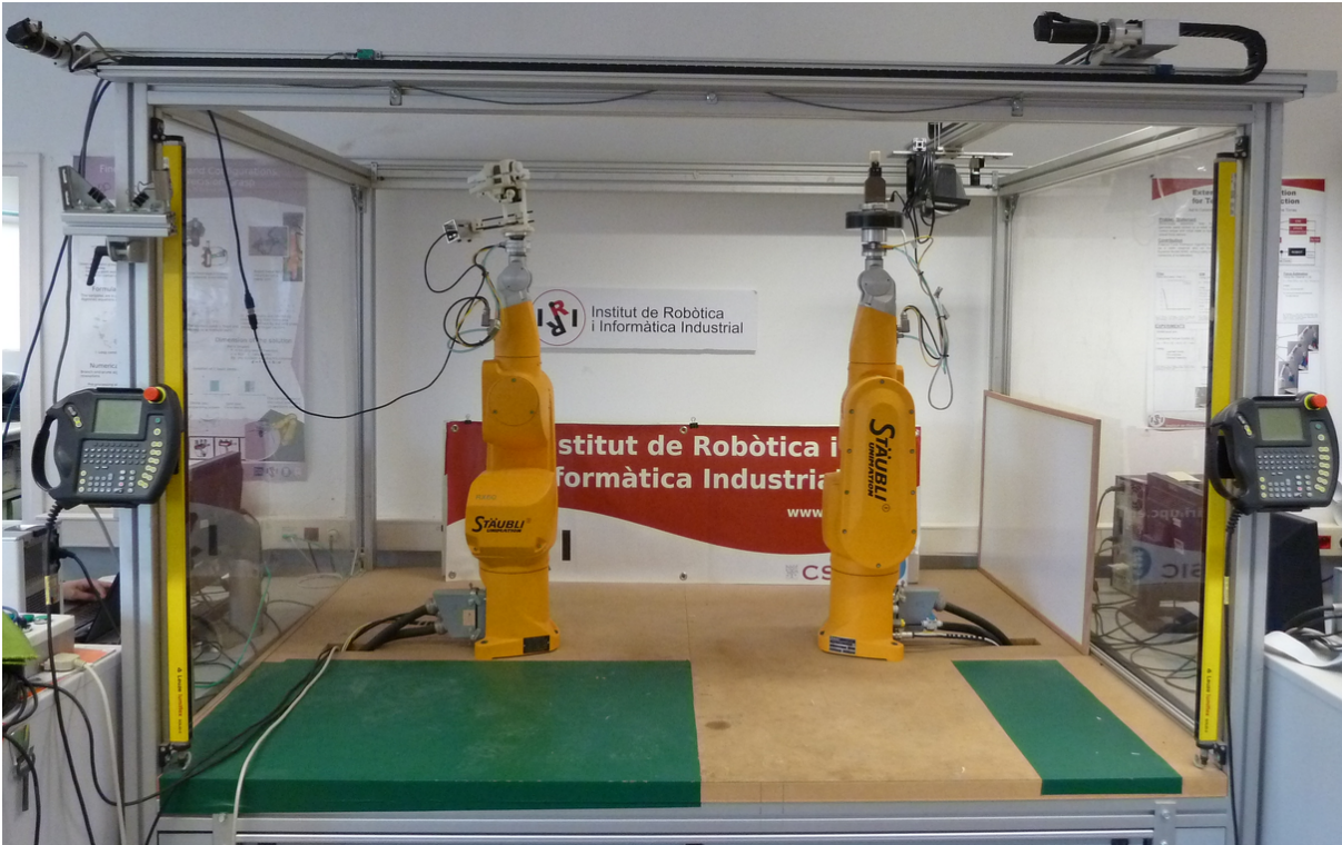
Figure 1: Picture of the actual Stäubli work-cell, with the two Stäubli RX60B robot at the center, and the XY robot at the top.
