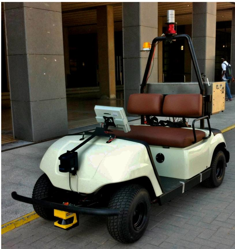
Figure 1: Picture of the real ackermann based robot available at the Mobile Robotics Laboratory at IRI.
