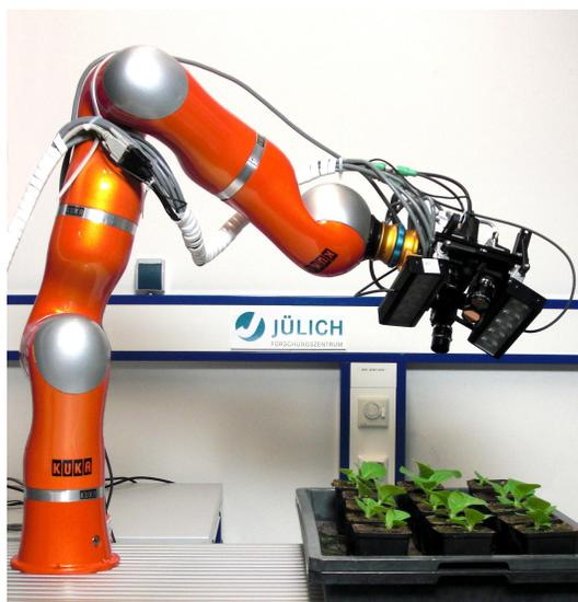
Figure 1: Robot gardener used in the European project GARNICS. A black-and-white 5 MP camera with infrared filter and required illumination devices were mounted on a lightweight KUKA LBR4 robot arm. For each tobacco plant the robot arm captured a stereo image pair from a top view at every hour.
