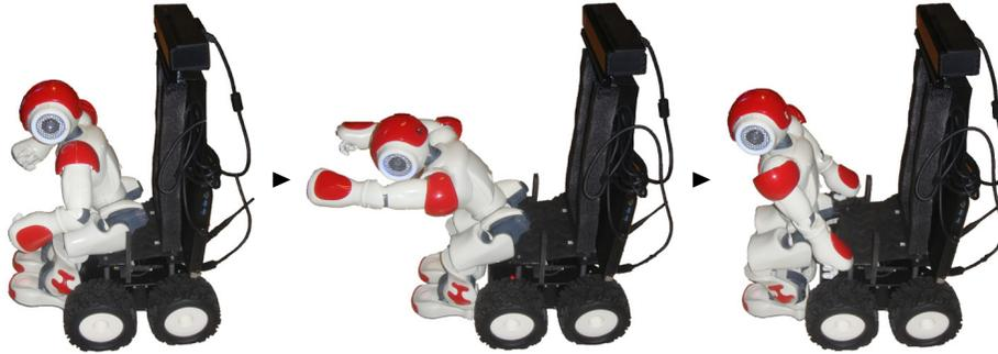
Figure 6: NAO's going down of the Wifibot to approach the object.
