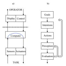
Figure 1: a) Model by (Sheridan, 1992), and b) Norman's modified model (Scholtz, 2003; Goodrich and Schultz, 2007) of interaction in a human supervisory control system.
