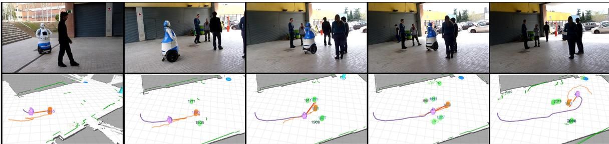
**Fig. 17 Real-life experiments 2:** A single robot companion experiment. *Top:* Dabo accompanying a person to a desired goal. *Bottom:* The same scene using the system interface.
