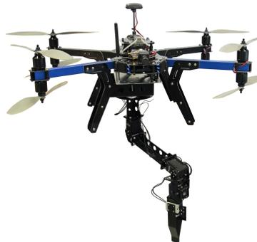
Fig. 1. Aerial manipulator, used in the experiments, consisting on a 3DR-X8 coaxial multirotor platform with a custom-built 3 degrees-of-freedom serial arm attached below.
