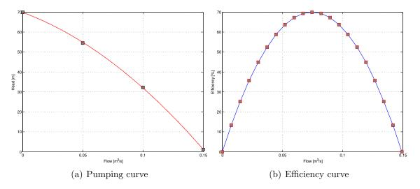
Figure 3: Pump characteristic curves
