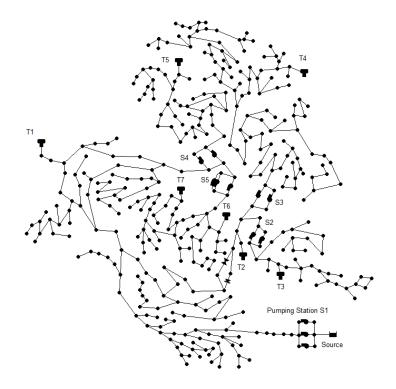
Figure 4: Original topology of the D-Town water network
