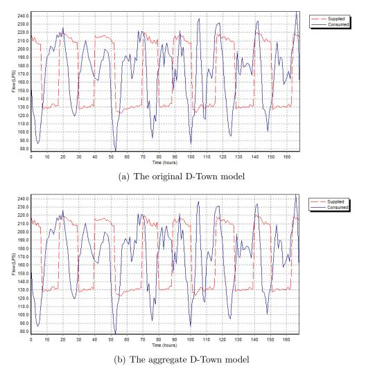
Figure 7: Validation of the produced and consumed system flows
