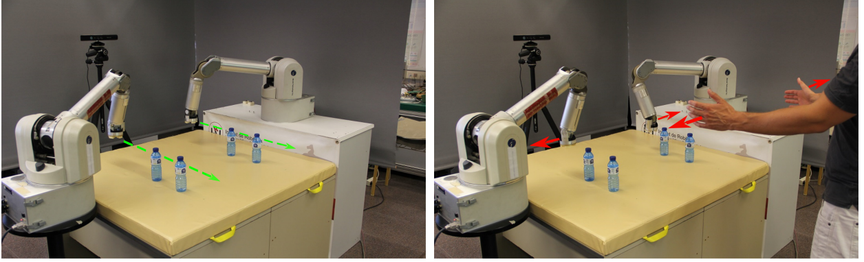
Figure 6: A user guiding a dual-arm robot by using hands’ gestures tracked by a Microsoft Kinect camera. The original robot trajectory is shown in green (left image). Red arrows show the user’s hands’ gestures and the corresponding robots’ motion in the teleoperation mode (right image).
