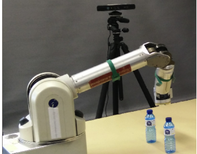
Fig. 1. The experimental setting consisting of a Barrett WAM robot arm and a Kinect camera.
