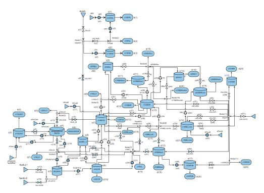
Figure 1: Barcelona DWSN aggregate diagram
