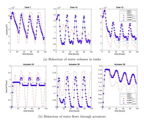
Figure 3: Comparisons of behaviours from selected tanks and pumps
