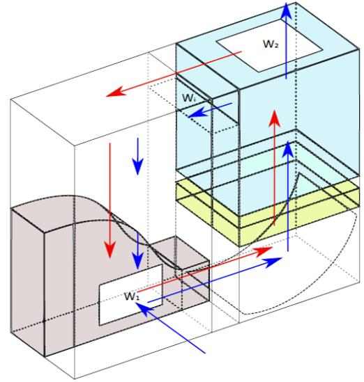
Fig. 1: Fuel cell air flows scheme
