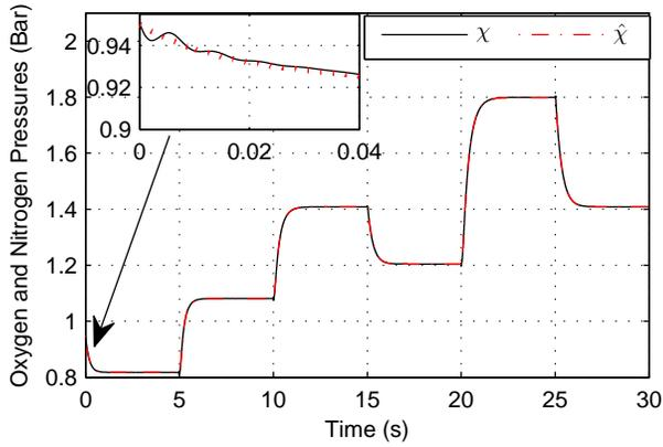
Figure 5: Estimation of  $\chi$  under stack-current variation
