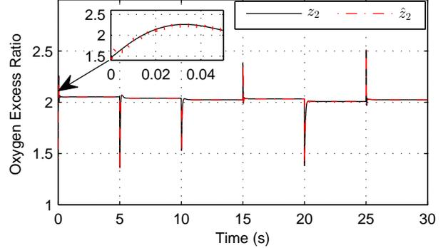
Figure 4: Estimation of  $z_2$  under stack-current variations
