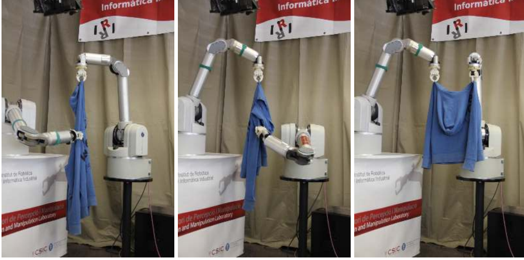
Figure 14: Process of bringing a garment to a target configuration. Initially, one robot arm grasps a jumper that is identified using the first CNN of the hierarchy. Then the garment is rotated until one of the pre-defined grasp points is predicted to be visible by the second CNN. Then a second robot arm approaches and grasps the jumper and moves it in front of the camera while the first arm moves away. Again, the garment is rotated until the first arm approaches the visible second pre-defined grasp point and moves the garment to the target configuration on the third image.
