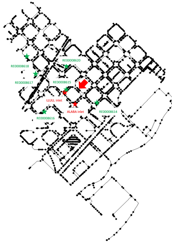
Fig. 2: The water network of Nova Icària district metered area (DMA) (EPANET model) highlighting inner pressure sensors (green stars), DMA inlets (red stars), and the exact location of the leak (red arrow) that was intentionally introduced to test the method.
