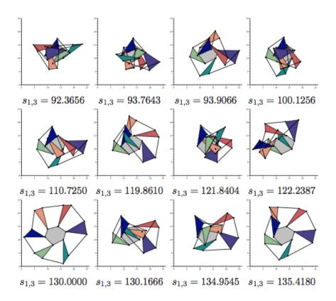
**Fig. 6** Some of the valid configurations of a 13-link Watt-Baranov truss. The position analysis of this mechanism using algebraic methods has been shown to be feasible when formulating the problem in terms of distance constraints [43].
