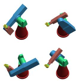
Fig. 2 The inverse kinematic problem of a serial robot consist in finding the robot configurations that position the end effector in a given pose. For the manipulator in the figure this problem has eight different solutions. Four of them are shown here.
