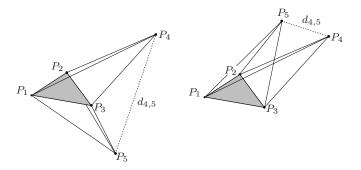
Fig. 7 Trilateration can be used to compute the distance between  $P_4$  and  $P_5$  from their distances to  $P_1$ ,  $P_2$ , and  $P_3$ , which form a fixed triangle. Two solutions are possible depending on the location of  $P_4$  and  $P_5$  with respect to the plane defined from points  $P_1$ ,  $P_2$ , and  $P_3$
