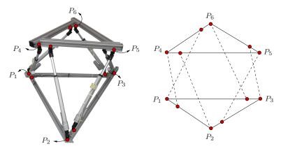
Fig. 9 Left: A hexapod structure. Right: Associated distance graph where nodes are points and edges are distance constraints. Solid lines denote distances that are constant independently of the configuration.
