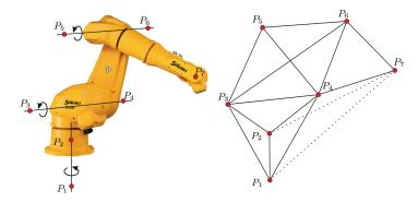
Fig. 10 Left: The configuration of the regional part of a wrist-partitioned 6R robot is determined by the location of seven points. Right: Associated distance graph where nodes stand for points and edges for known distances between the corresponding points. Solid lines represent constant distances, regardless of the location of the end-effector.
