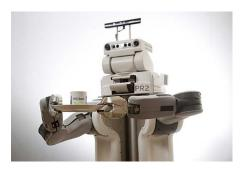
Fig. 15 A two-armed service robot holding a plate. The arms must be in contact with the plate and the plate must remain horizontal to avoid tilting the coffee mug on it. A loop of kinematic constraints is thus generated.
