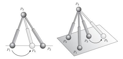
Fig. 14 Singularity invariant leg rearrangements. Left: Rearrangement along a line connecting two anchor points. Right: Rearrangement in a plane defined by three anchor points.
