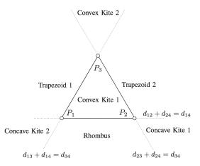
Fig. 11 Taking triangle  $P_1$ ,  $P_2$ , and  $P_3$  as a reference, the plane is divided in seven regions. If  $P_4$  is bound to be in one of these regions,  $s_{3,4}$  is monotone with respect to the rest of squared distances. The boundaries separating the monotonic regions correspond to configurations where there is an alignment of three points.
