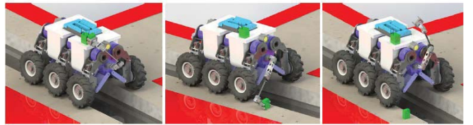
Fig. 3. SIAR Robot deploying one wifi communication repeater.
