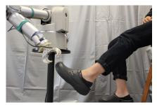
(a) Approach action, to get closer to the (b) Insert shoe action, using an elaborated wrist rotation (see supplementary video).
