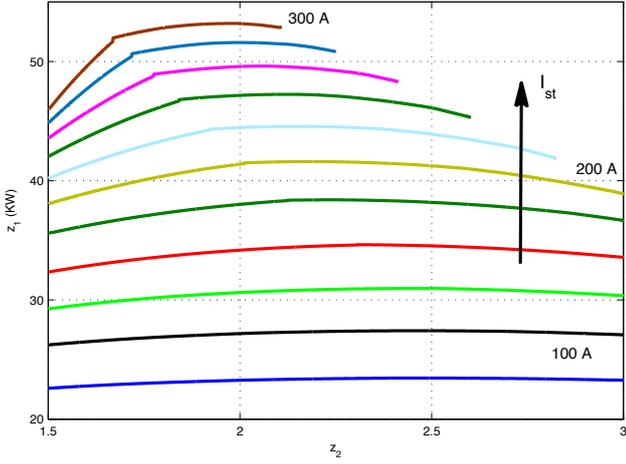
**Fig. 2:** Fuel-cell system performance under different stack-currents
