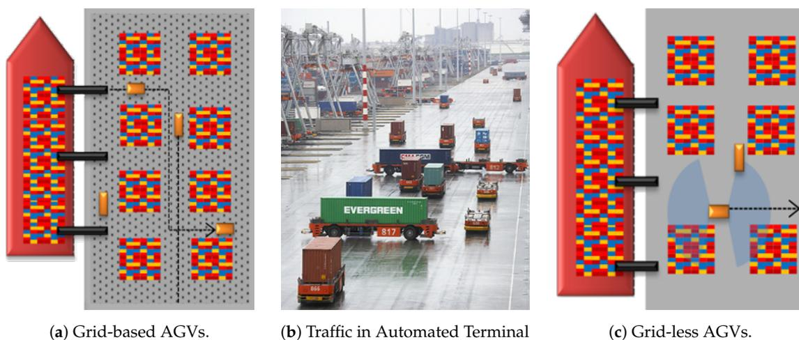
**Figure 1.** Representation of a current automated port terminal (a) and the aimed next generation grid-less AGVs (c). Vessels arrive at the seaside of the port and the cranes unload or load the containers. AGVs move the containers from the cranes area to the stacking area represented here with multi-color squares. Presently, AGVs follow pre-defined paths which limit their movements (a,b). Grid-less AGVs will provide vehicles with decision capacity and freedom of movement as seen in (c).
