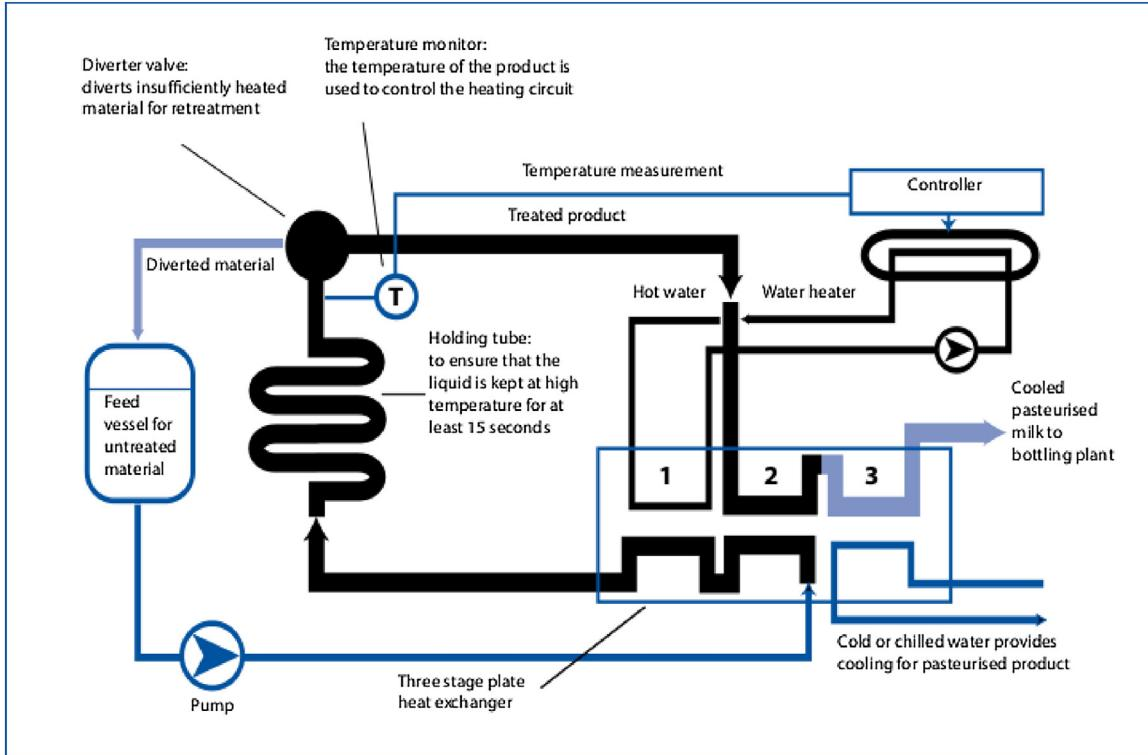
**Fig. 1.** Conceptual diagram of the pasteurization plant.
