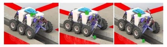
Fig. 2. SIAR Robot deploying one wifi communication repeater.
