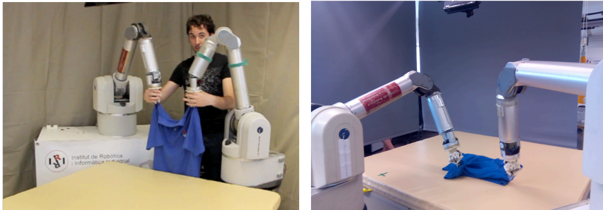
FIGURE 2. Experimental scenario of the task of teaching a bimanual robot to fold garments, in this case a polo shirt, by means of an initial demonstration (left) followed by autonomous learning for reinforcement (right).
