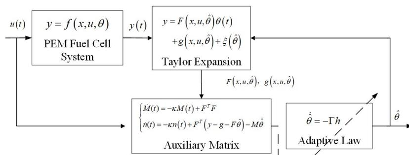
Figure. 1. Structure of the proposed parameter estimation scheme
