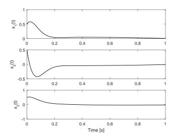
Fig. 3. Closed-loop state trajectories  $(x_0 = [0.5, 0.5, 0.5]^T)$ .
