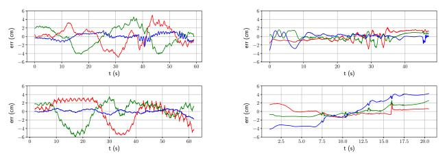
Fig. 6: Translation estimation error (cm) as a function of time (s). In the clock-wise sens, starting from the top-left corner, the datasets are handheld camera, stairs climbing, stairs descending and walking on flat ground. RGB colors correspond to xyz axes.
