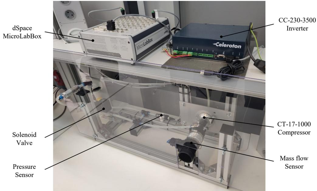
Figure 11: Hardware setup
