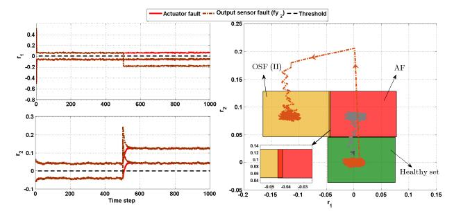
Figure 11: FD results when the obtained magnitude using MDF is considered for the case of occurrence of  $f_{y_2}$  and  $f_a$  at the same time (AF denotes the residual set when simulation actuator fault  $f_a$ ).
