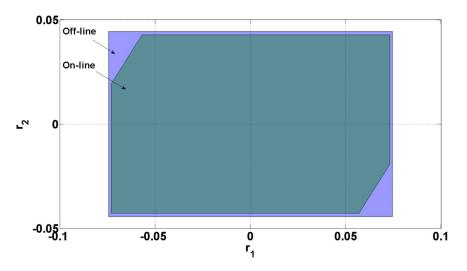
Figure 5: Comparison of the residual set using on-line and off-line approaches in steady state.
