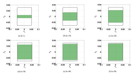
Figure 4: On-line propagation of residual set using zonotopic IOA during transient state and healthy operation of the system.
