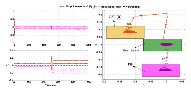
Figure 10: Always separable (ISF and OSF (II) denote the residual set when simulation input sensor fault  $f_u$  and output sensor fault  $f_{y_2}$ , respectively).
