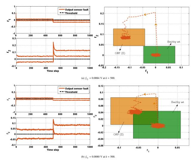
Figure 8: FD results in the case of occurrence of the sensor fault  $(f_{y_2})$  during steady state, i.e., k = 500.
