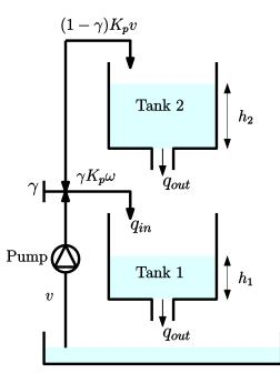
Figure 2: Schematic diagram of the Two-tanks system.
