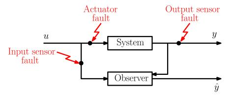
Figure 1: Graphical interpretation of the different actuator and sensors faults.
