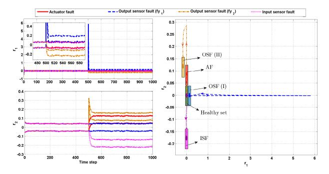
Figure 13: FD results when the maximum magnitude that obtained using MIF analysis in Table 2 for each type of faults is simulated.
