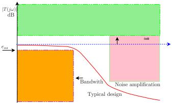
Fig. 3. Complementary Sensitivity function specifications over the Bode diagram.
