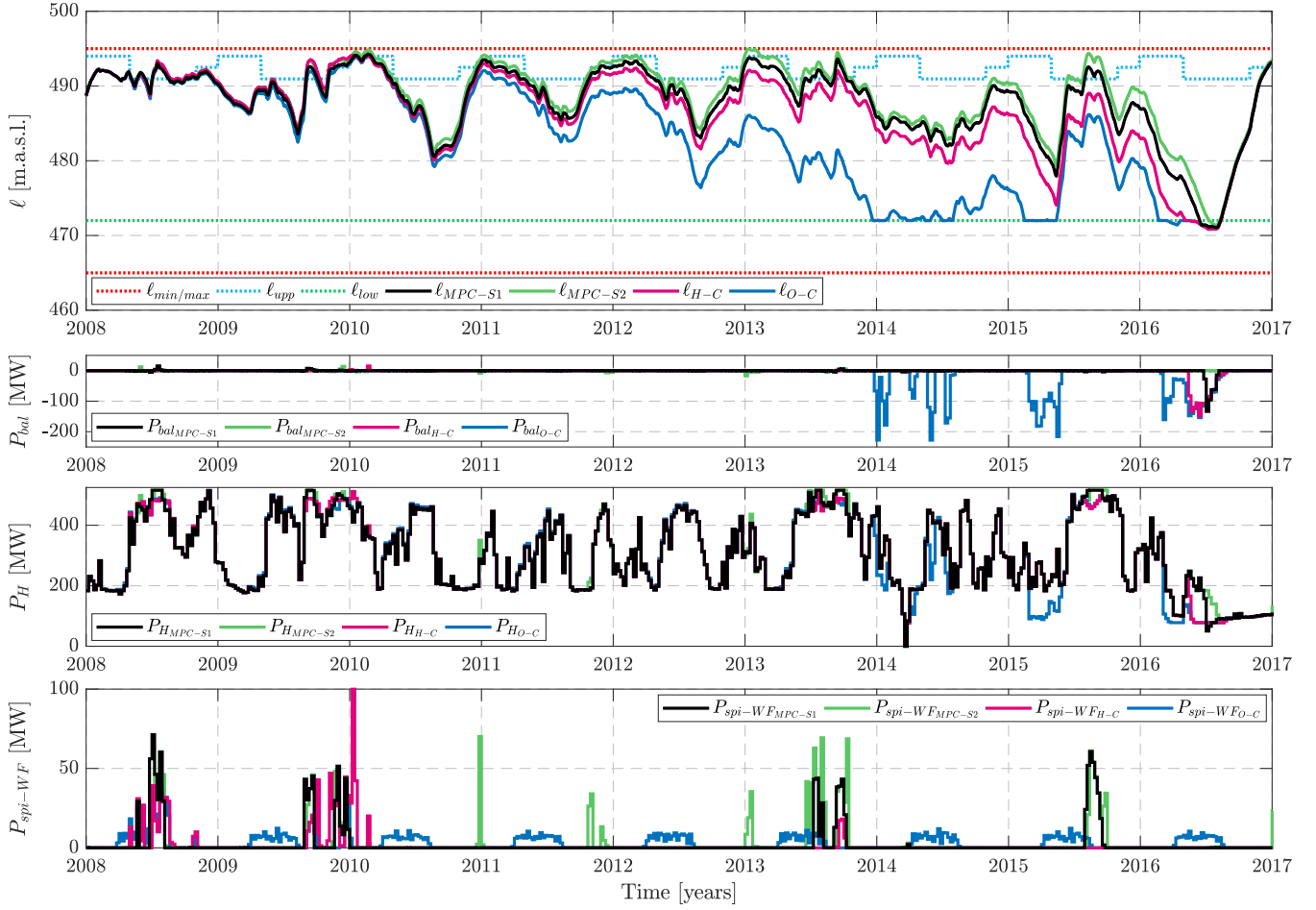
Fig. 9: O-C (blue), H-C (magenta), MPC-S1 (black) and MPC-S2 (green) nine year simulation. 1st : Reservoir levels, minimum and maximum levels (dotted-red), upper threshold (dotted-sky blue) and lower threshold (dotted-green). 2nd : Weekly average balance between generated and demanded power. 3rd : Weekly average HPP dispatch. 4th : Weekly average wind power spillage.
