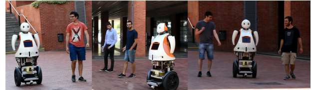
Figure 1. Real-life experiments in the Barcelona Robot Lab. Left: Our robot, named Tibi, accompanies one volunteer using the adaptive side-by-side [26]. Center: Tibi accompanies the volunteers at the lateral of the side-by-side [27]. Right: Tibi accompanies the volunteers at the middle of the Side-by-side formation [27].
