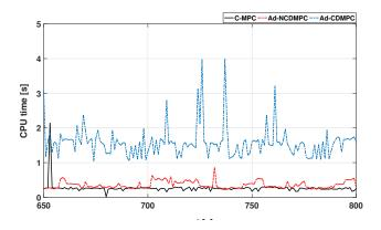
Figure 10: CPU time spent by iteration to find an optimal solution by using centralised and non-centralised control architectures.
