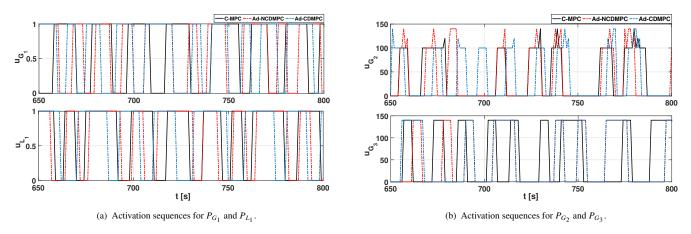
Figure 7: Optimal activation sequences of peripheral devices by using centralised and non-centralised control architectures.
