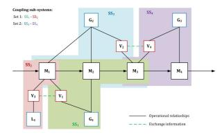
Figure 6: Proposed sub-systems division for the four-stage serial process line in Figure 3.
