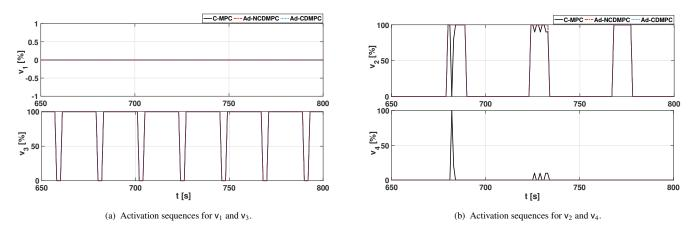
Figure 9: Optimal activation sequences for the aperture of valves by using centralised and non-centralised control architectures.
