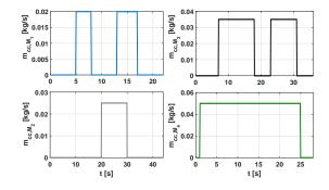
Figure 5: Sequences for the coolant consumption from machines in the fourstage process line along  $T_{M_i}$ .
