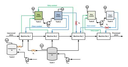
Figure 3: Four-stage serial process line with four peripheral devices.
