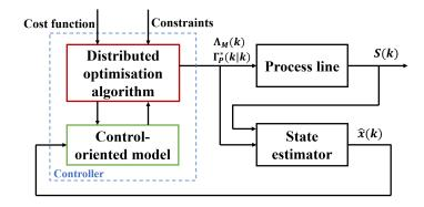
Figure 2: Proposed control scheme to minimise the energy consumption of a manufacturing process line.
