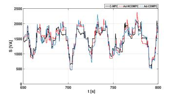
Figure 8: Energy consumption profile obtained by using centralised and noncentralised control architectures.
