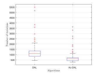
Fig. 4. The number of iterations performed by each algorithms. The blue boxes show the  $25^{\text{th}}$  percentiles until the  $75^{\text{th}}$  percentiles, the red lines show the median, and the + symbols indicate outliers.
