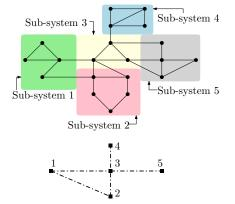
Fig. 1. An example of a small-scale energy network. Top figure shows graph  $\mathcal{G}$  where the nodes in  $\mathcal{N}$  are depicted as dots and the links in  $\mathcal{E}$  are depicted as solid lines. The graph  $\mathcal{G}$  is partitioned into five subsystems. Bottom figure shows graph  $\mathcal{G}^{s}$  where the subsystems in  $\mathcal{P}$  are depicted as filled squares and the links in  $\mathcal{E}^{s}$  are depicted as dash-dotted lines.
