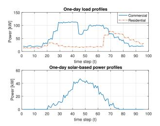
Fig. 3. One-day residential and commercial load profiles (top plot) and oneday solar-based power generation profile (bottom plot).
