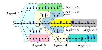
Fig. 2. The locations of non-dispatchable units (indicated by filled squares,  $\square$ ), dispatchable generators (indicated by empty squares,  $\square$ ), and storage units (indicated by crosses,  $\times$ ) in the PG&E 69-bus distribution network, which is partitioned into eight subsystems [29].
